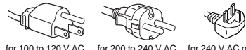
for 100 to 120 V AC for 200 to 240 V AC for 240 V AC only
